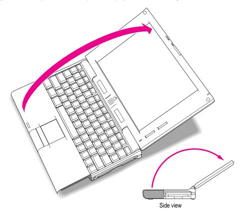
7 Set the computer down and open the display to its maximum angle.
